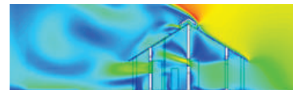
Fig | 36: Elevation View of Wind from South - Single Storey House
