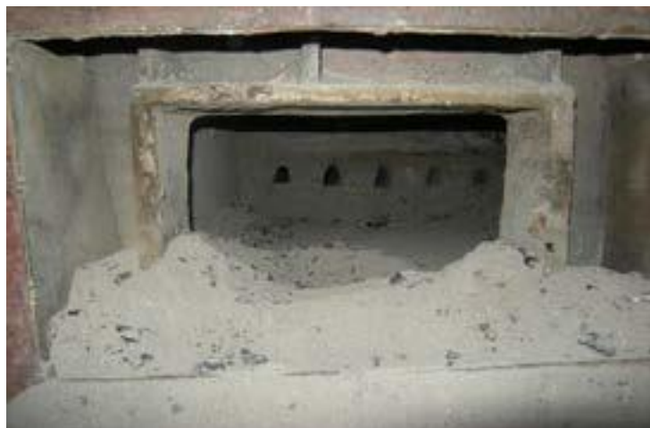
Figure 2: Photograph showing a large quantity of ash collected, probably due to long hours/days of work
