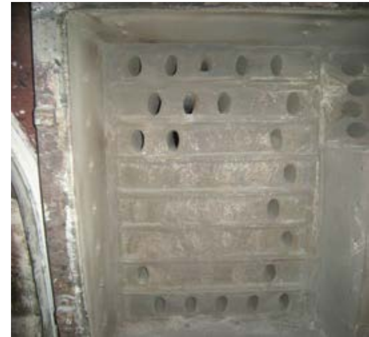
Figure 3: Photograph showing blocked oval tubes
