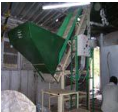
Figure 4: Belt conveyor and controlling system
