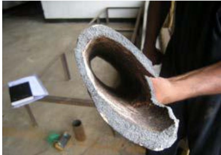
Figure 1: Photograph showing uneven thickness of an oval tube
