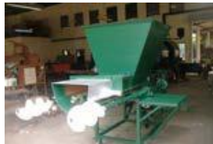
Figure 6: Two side screws maintain the fuel bed thickness
