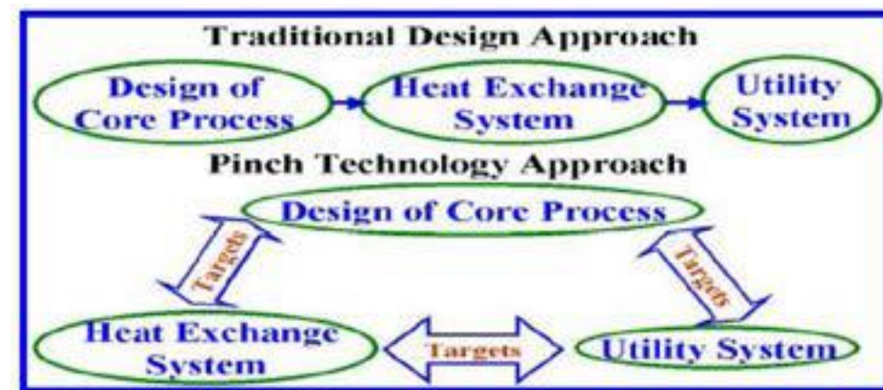
Figure 2: Graphical Representation of Traditional & Pinch Design Approaches (Source – Reference [4])
