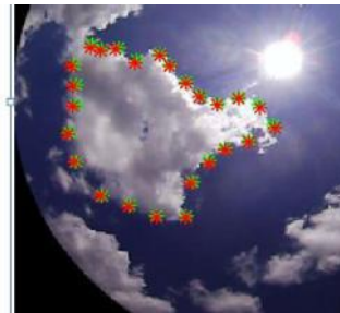
Figure 6: Feature points in the first image (Red) corresponding feature points in next image (Green)
